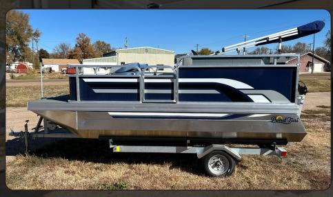
The 14 Series is the largest model in the Pond-Tini fleet with an 8 person capacity. It's rated for up to 40HP, yet still light enough for electric only motors.
